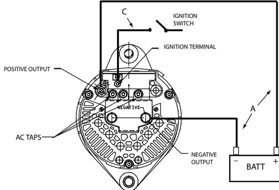
**4800/4900 Self Excite Wiring Diagram**
