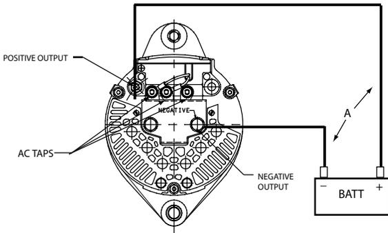
**4800/4900 Remote Voltage Sense and Lamp Driver Wiring Diagram**
