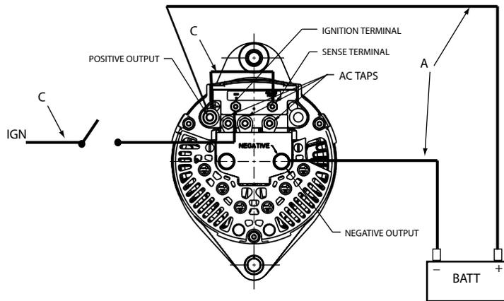
Wiring for battery isolator applications.
